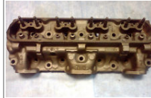
7M5 CYLINDER HEAD GM 1972 455cid PONTIAC GTO P/N: 494998 2.11/1.77 114cc
