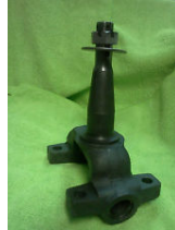
Spindle - Fits 1957 Chevrolet Truck with Drum Brakes Stock Height w/ Castle Nut
